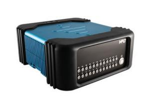
Built on the latest MicroPulse technology, the MPLT takes the LT concept to a new level. The MPLT is a compact and completely enclosed unit (no fans). Using Power over Ethernet technology, Gigabit Ethernet for seriously fast data transfer, including extended dynamic range modes and with up to 48 conventional channels in its standard enclosure. Ideally suited for multi-probe pulse-echo and TOFD inspections requirements.
